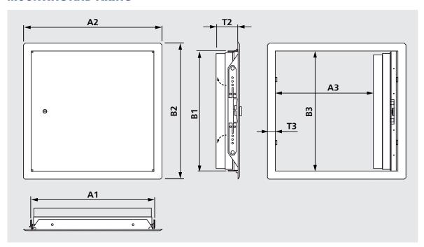
Clearance dimensions: A3 - 15 mm (from 500 x 500) x B3 Aperture dimension: Installation dimension A1 + 5 mm x B1
